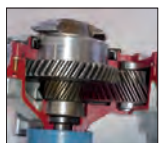
Gear transmission running in oil
