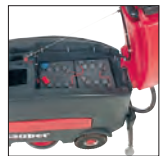
Machine open showing the batteries
