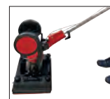
Turn the handle completely upside down to get max. weight on the ground
